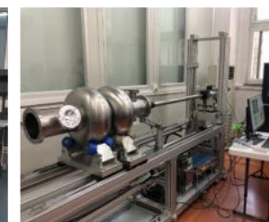
Cavity inspection camera and grinder
