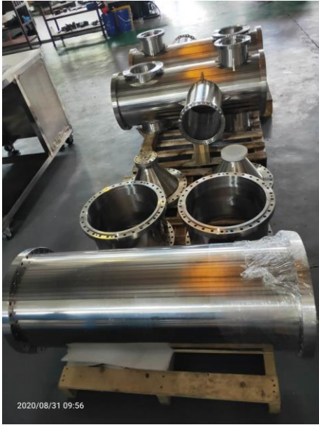
Vacuum chamber Components
