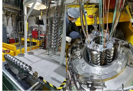
Booster 1.3GHz 9 cell cavity
