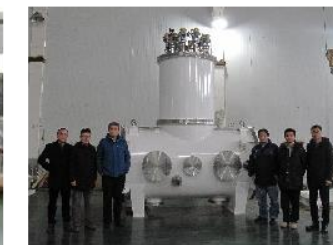
Horizontal test cryostat
