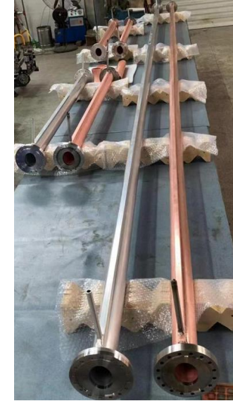
Two 6m long vacuum chambers both with copper and aluminum
