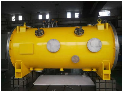
Cryomodule vacuum vessel and cold mass
