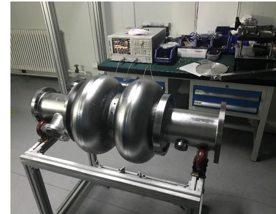
Collider ring 650Mhz 2 cell cavity
