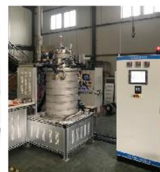
Nb 3 Sn furnace
