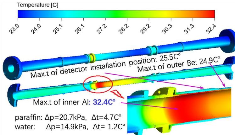
**Central beampipe** made with **Beryllium** and located at  $r = 14 \text{ mm}$ , beampipe opened up in the forward region and made with aluminum
