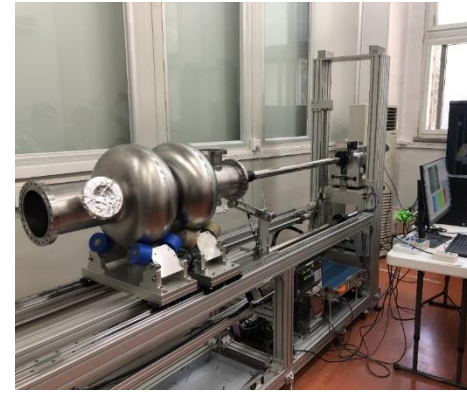
Cavity inspection camera and grinder
