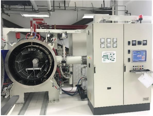
Vacuum furnace (doping & annealing)
