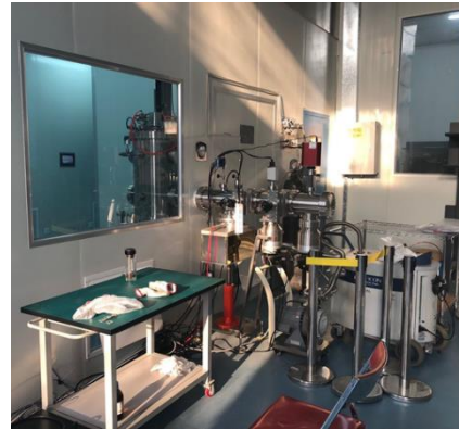
Nb/Cu sputtering device
