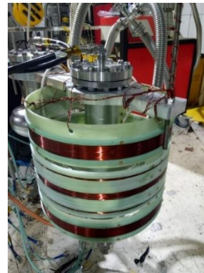
Helmholtz coil for cavity vertical test
