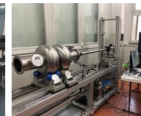
Cavity inspection camera and grinder
