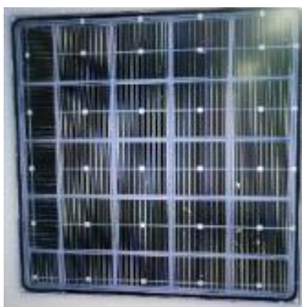
IHEP-NDL LGAD-V2 Pixel size 1.3 \times 1.3 mm 2
