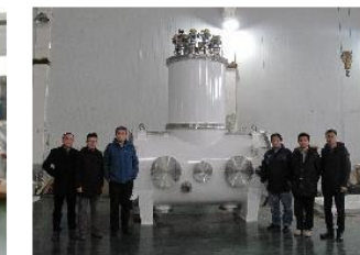
Horizontal test cryostat
