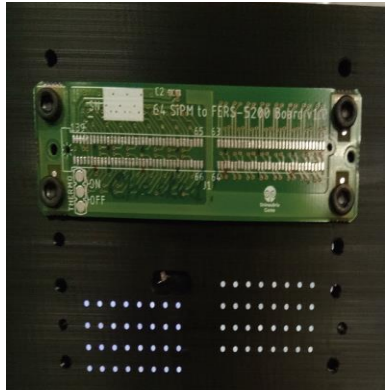
160 scint. fibers 160 Cherenkov fibers Tower: 20 rows x 16 columns
