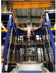
Klystron No. 1 Efficiency 65% (2020)
