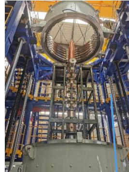
Klystron No. 2 Efficiency 77% (2021)
