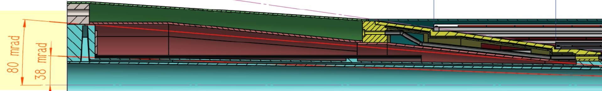
**Al pipe  $x = 200 - 700 \text{ mm}$ , inner  $0.5 \text{ mm}$ , outer  $0.35 \text{ mm}$  thick**
