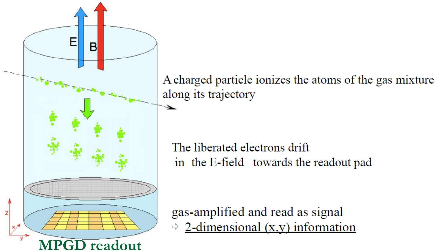
z component is obtained from drift time ⇒ 3-dimensional (x, y, z) information
