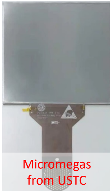
Kapton-based low-bkg front end electronics
