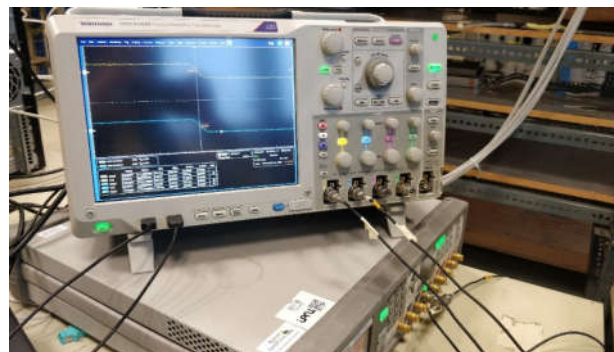
Oscilloscope confirms the output of the signal generator
