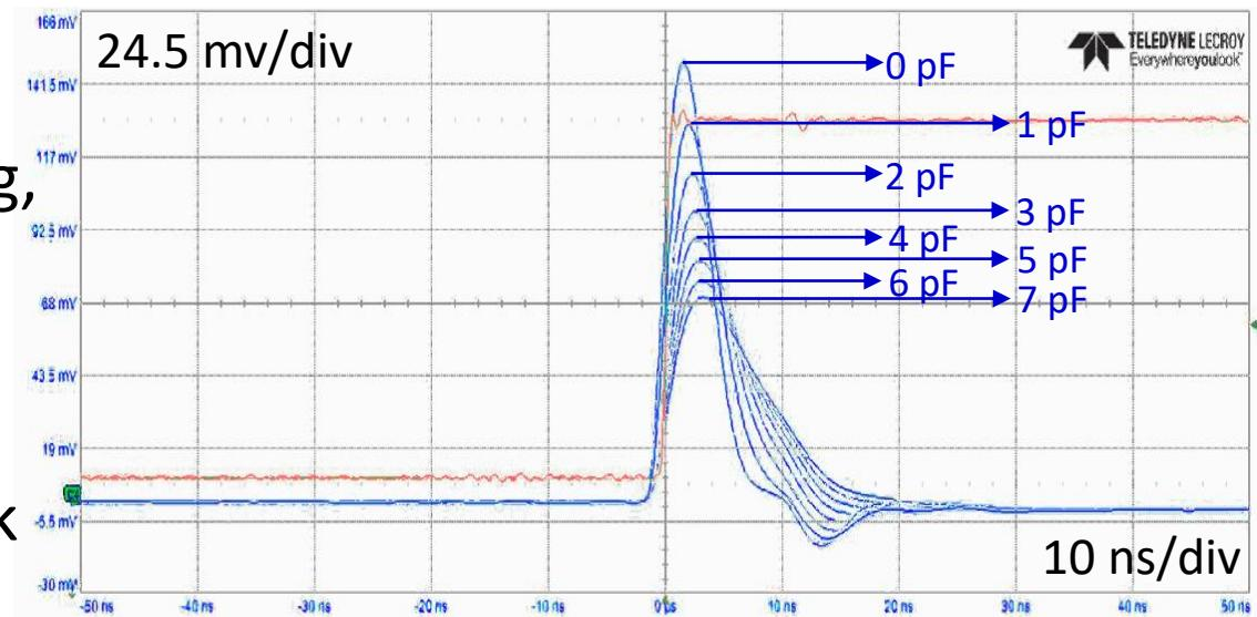
Waveform at different input capacitance 0~7 pF, input charge 10 fC
