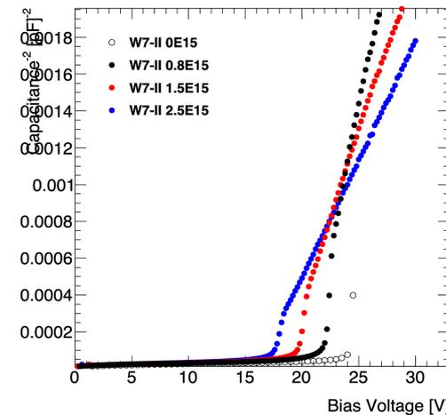
$V_{gl}$  after different radiation dose
