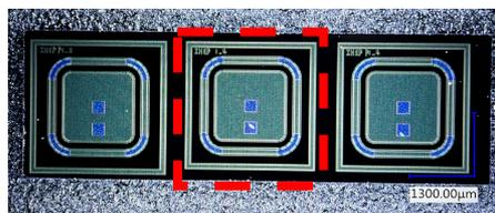
Test unit including a LGAD sensor and two PIN sensors
