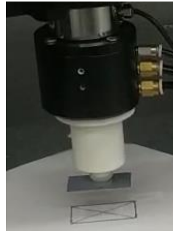
Placing dummy sensor
