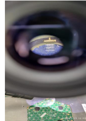
Wires in a real 6-inch module
