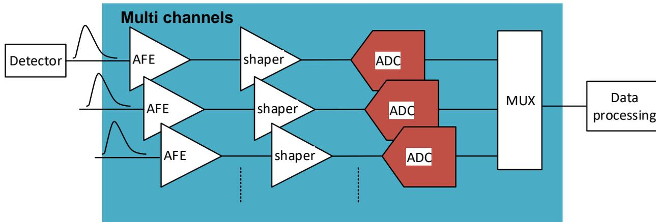
Signal chain in readout electronics
