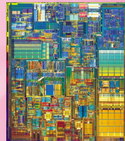
Intel Pentium 4 (2000) 42M transistors, 1.5GHz
