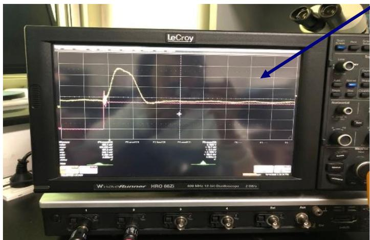
Analog output of a pixel @  $V_{in} = 0.9 \text{ V}$
