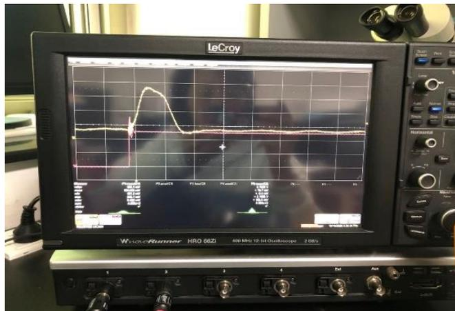
Analog output of a pixel with a **voltage input**
