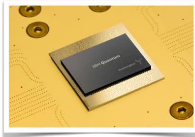
IBM Quantum Hummingbird (65 qubits)
