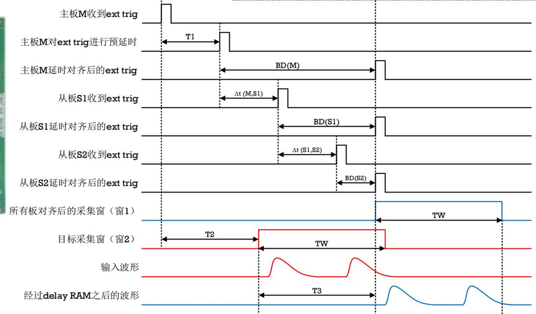
$$T_{relative3} = T_3 - T_{ext} + T_{B1/B2} + T_{B2/B3}$$
