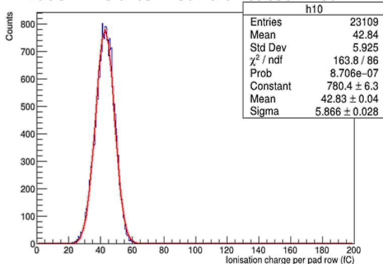
$$\text{separation power} = \frac{dE / dx(A) - dE / dx(B)}{\sigma(dE / dx)_{A,B}}$$
