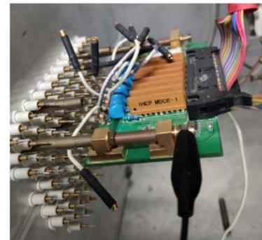
➔ Readout by an oscilloscope that connects to the preamplifier with a 18m cable
