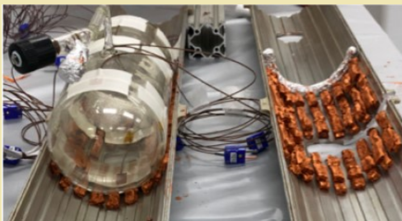
Figure 3: "Packing" a 2-liter cell into an aluminum shell using copper-based thermal grease.
