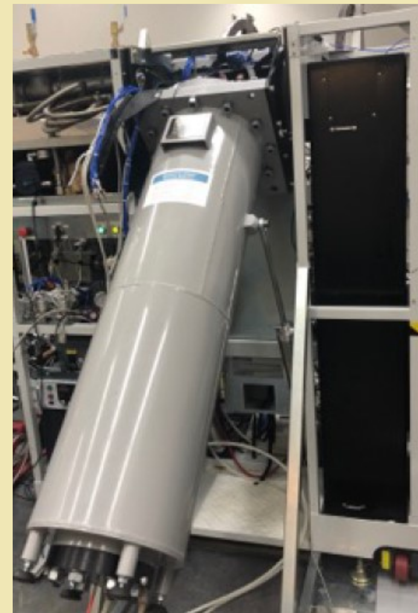
Figure 5: Zeppelin-4 helium-3 polarizer (4th generation) with the pressure vessel containing SEOP cell, tilted at 45 degrees. Left side of the frame contains gas panels, oil pumps, electrical, while the laser box (black) is located on the right side. The pressure vessel is made of steel and rated for up to 20.7 atm. An pressure interlock system automatically adjusts the pressure to match the cell. It includes a full length solenoid for B0 magnetic field. An additional mu-metal liner was added for increasing uniformity. Polarizer has casters and can be re-located.
