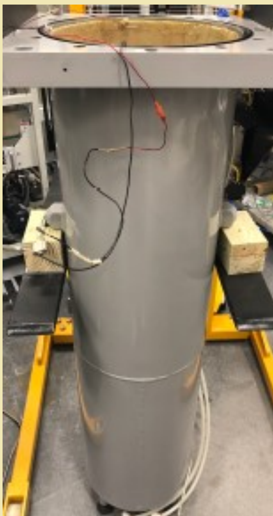
Figure 5: Zeppelin-4 helium-3 polarizer (4th generation) with the pressure vessel containing SEOP cell, tilted at 45 degrees. Left side of the frame contains gas panels, oil pumps, electrical, while the laser box (black) is located on the right side. The pressure vessel is made of steel and rated for up to 20.7 atm. An pressure interlock system automatically adjusts the pressure to match the cell. It includes a full length solenoid for B0 magnetic field. An additional mu-metal liner was added for increasing uniformity. Polarizer has casters and can be re-located.
