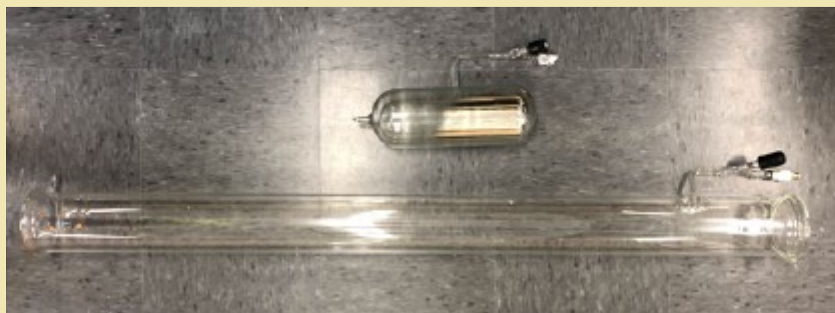
Figure 2: Examples of 2-liter cell (~30cm) and 8-liter cell (~120cm), loaded with a 5:1 (by mass) K-Rb alkali mix, and with side glass valve.
