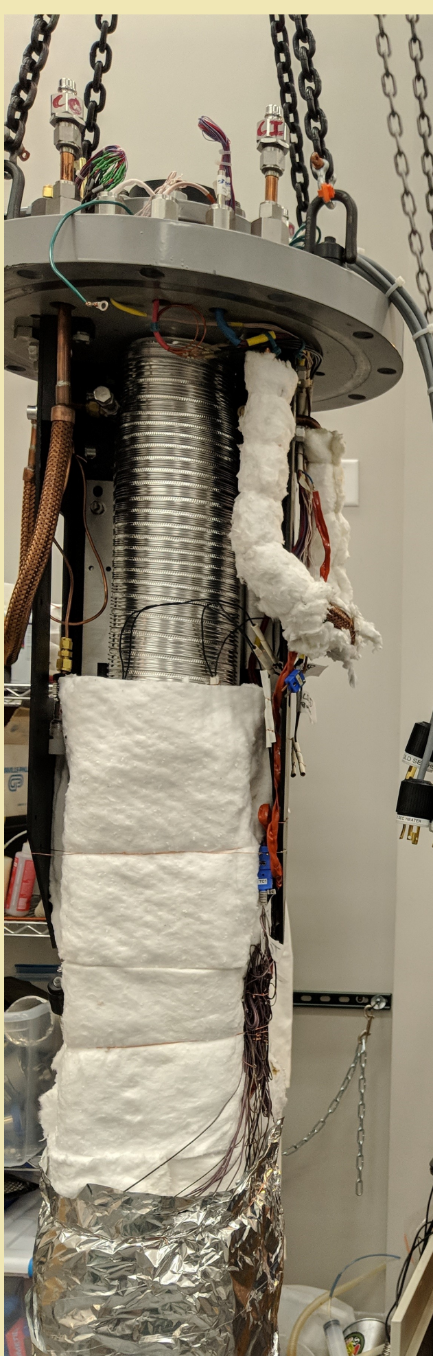
Figure 3: "Packing" a 2-liter cell into an aluminum shell using copper-based thermal grease.
