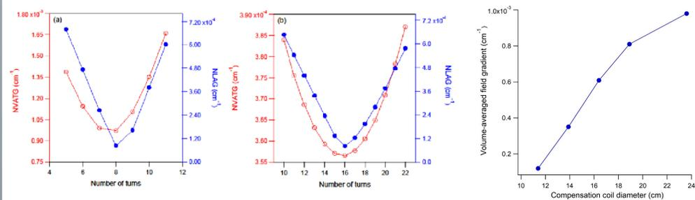
Normalized line-averaged gradients (NVATG)  $|\partial B_z/z|/B$  and NVATGs were calculated as a function of the number of turns of the compensation coil for a cylindrical  $^3\text{He}$  cell 12 cm in diameter and 10 cm long for the hole compensation configurations. The normalized linear-averaged gradients (NLAG) minimizes at the same location as the NVATG. This shows that the NLAG can be used a direct evaluation criterion for minimizing the NVATG when experimentally optimizing a MSS.
