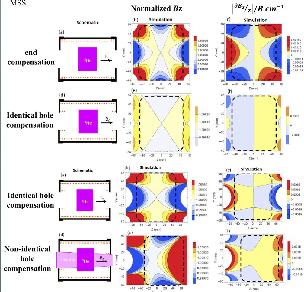
NVATG is  $9.8 \times 10^{-4}\text{ cm}^{-1}$  and  $1.2 \times 10^{-4}\text{ cm}^{-1}$  for the end compensation and identical hole compensation, respectively. This indicated an improvement in the NVATG by a factor of 8.2 for the identical hole compensation compared to the end compensation.
