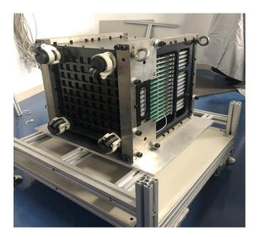
The Sci-ECAL was used LED driver to monitor the SiPM gain day by day
