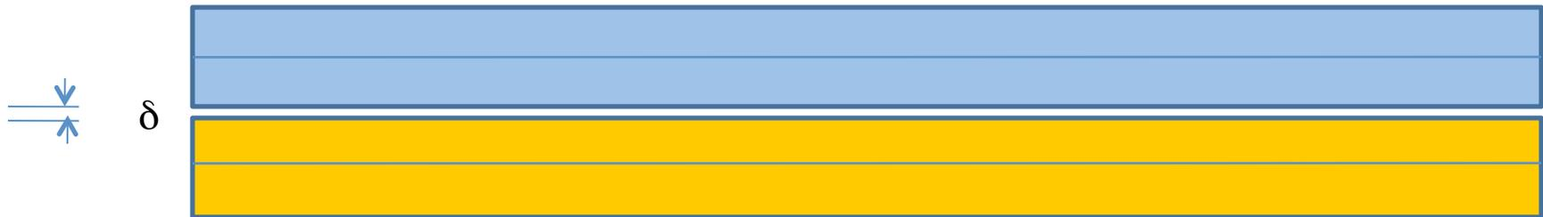
Method: Use two 1 mm spacing MWPC horizontal wire planes upstream of the strip scintillator counters to measure the vertical position of beam tracks that pass through the scintillator strips. Take data as the beam ( $\sim 1\text{cm}$ ) scans the crack.
