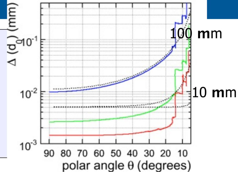
Impact parameter resolution vs polar angle of shallow tracks
