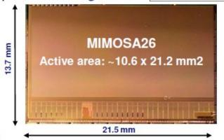
Lab. and beam tests: 62 chips tested, yield ~75%
