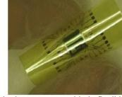
Fully functional microprocessor chip in flexible plastic envelope. Courtesy of Piet De Moor, IMEC company, Belgium
