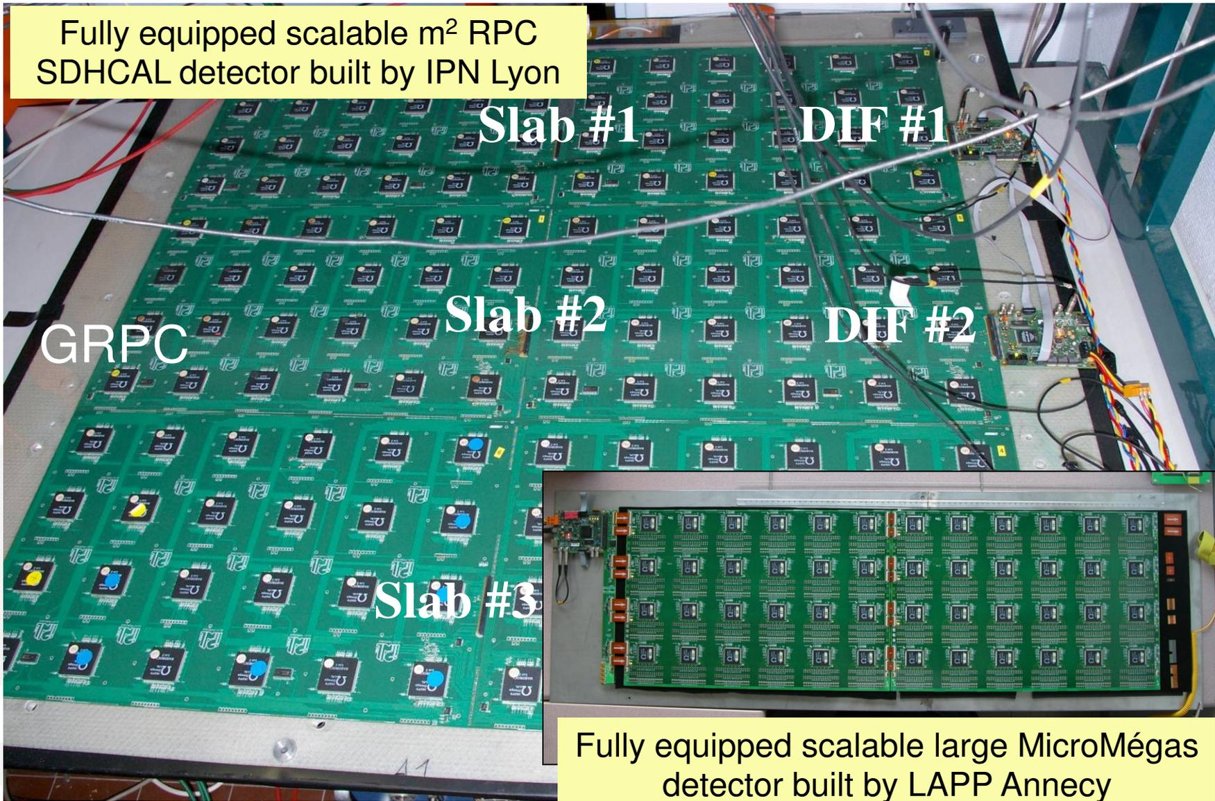
Fully equipped scalable m<sup>2</sup> RPC SDHCAL detector built by IPN Lyon
