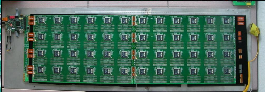
Fully equipped scalable large MicroMégas detector built by LAPP Annecy
