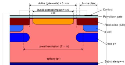
Figure 4. Channel cross section.
