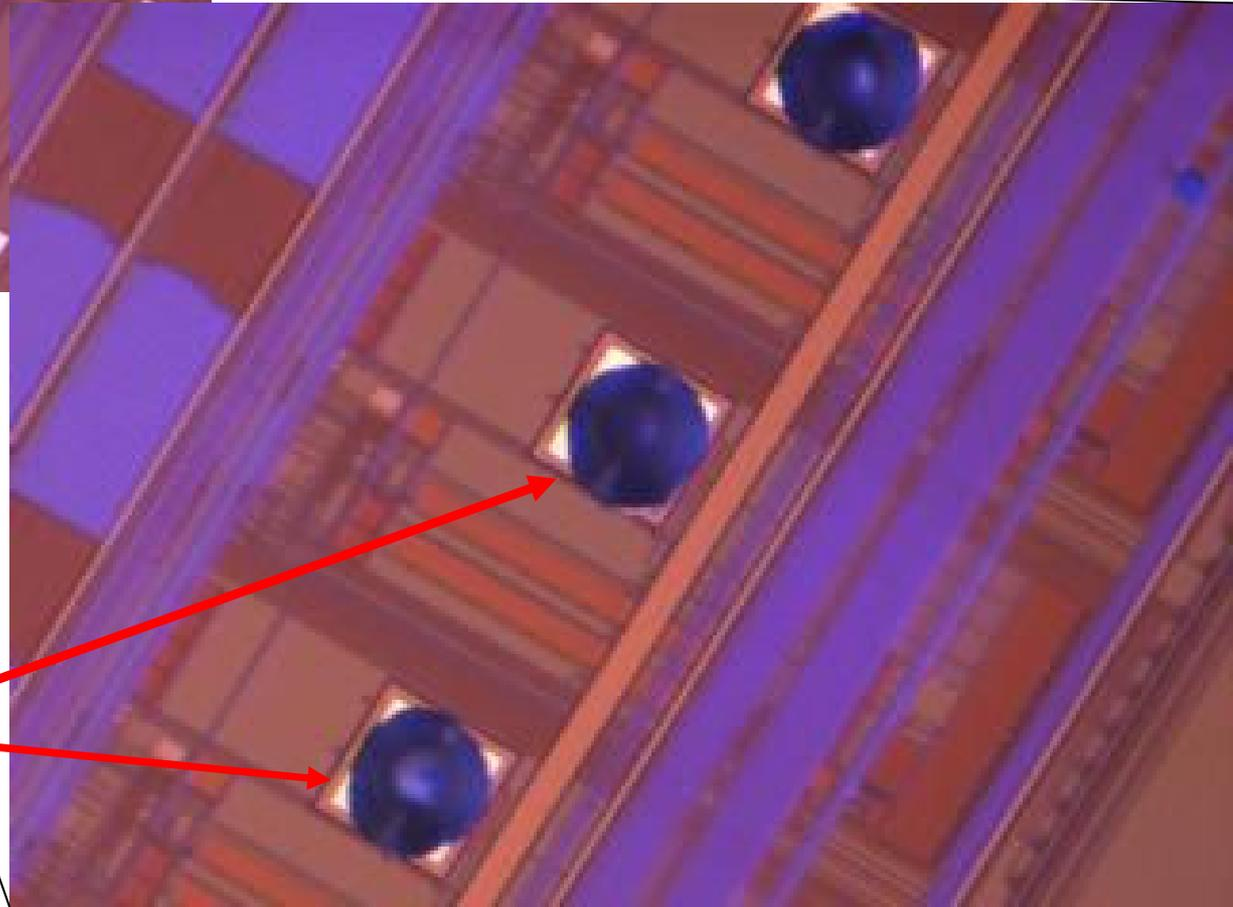
Studs are well-formed and centered on the  $70 \times 70 \mu\text{m}$  pads.
