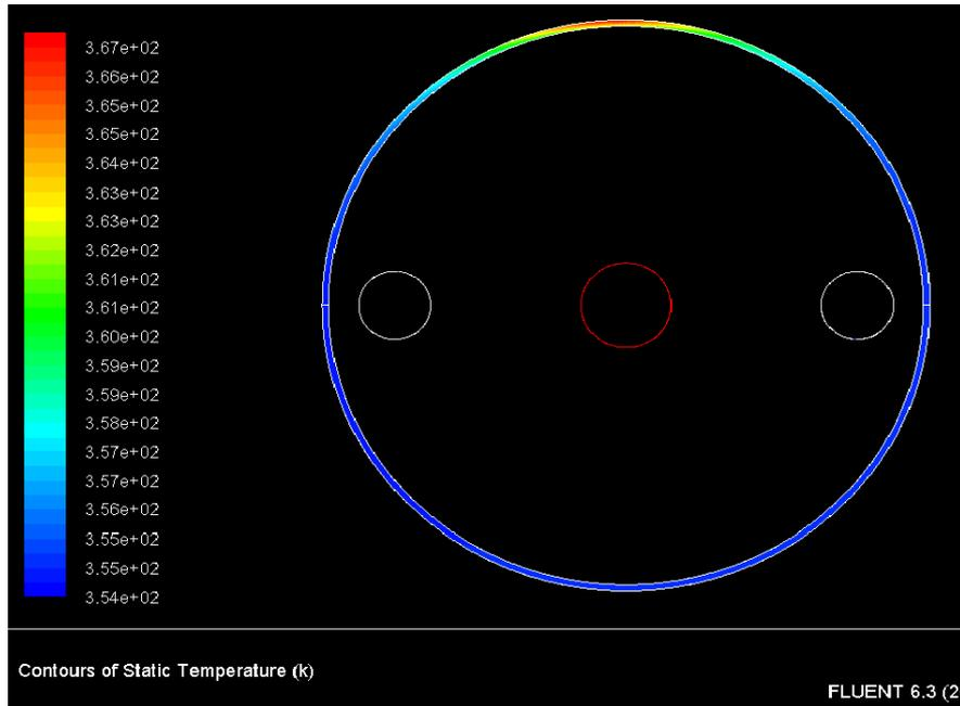
max vessel temperature -  $94^{\circ}\text{C}$
