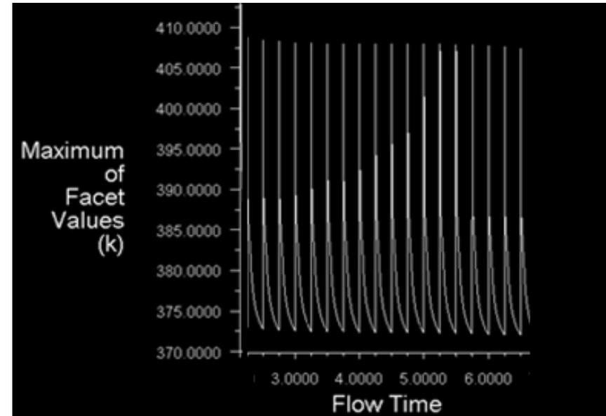
Maximum temperature  $\sim 135^{\circ}\text{C}$  and variation with time  $\sim 36^{\circ}\text{C}$
