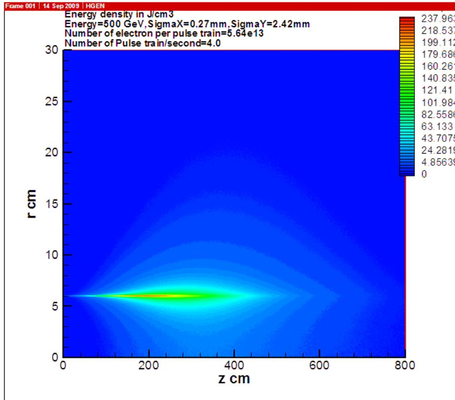
Energy deposited by one bunch train in the water (beam travelling along z-axis) max @ z=1.8m
