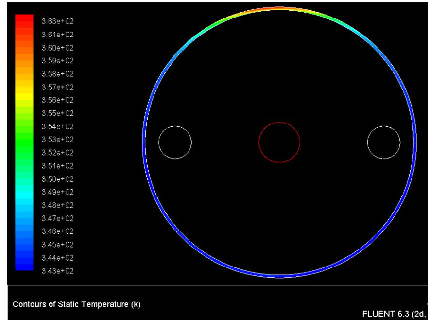
max vessel temperature -  $90^{\circ}\text{C}$
