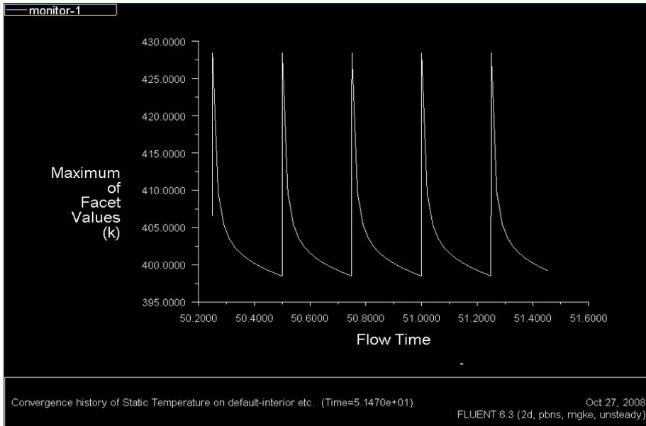
Maximum temperature  $\sim 155^{\circ}\text{C}$  and variation with time  $\sim 30^{\circ}\text{C}$
