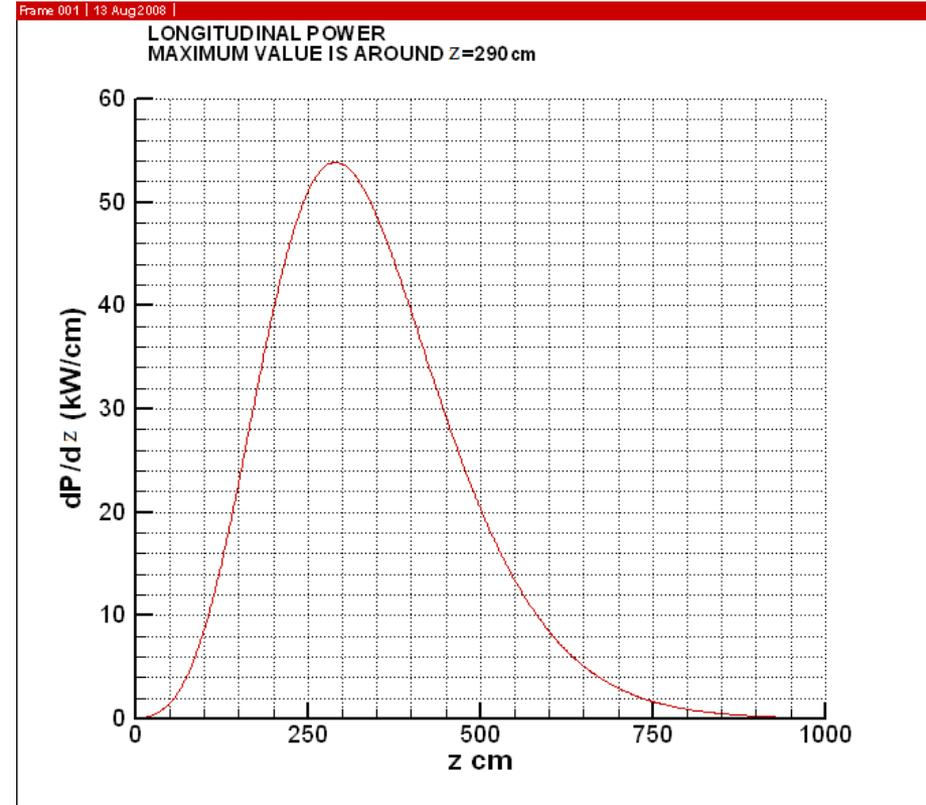
Radially integrated longitudinal linear power density max @ z=2.9m
