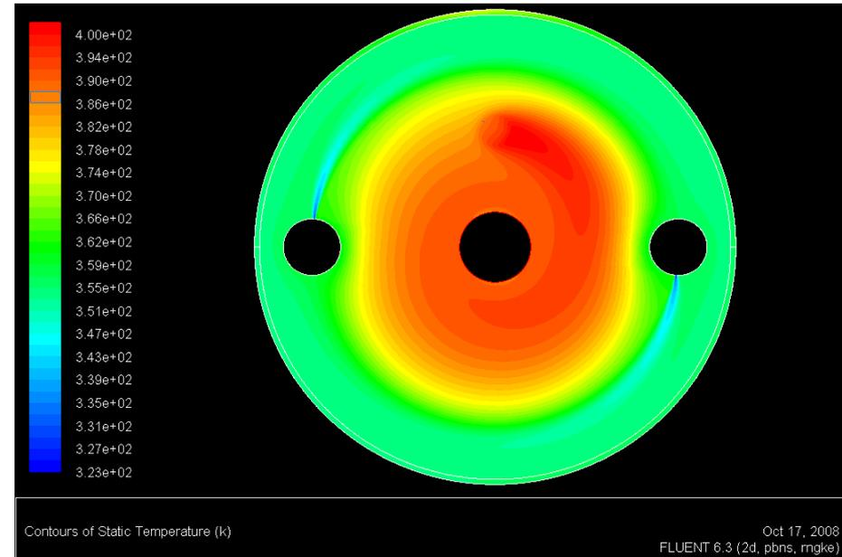
Steady state temperature distribution at  $z = 2.9\text{m}$
