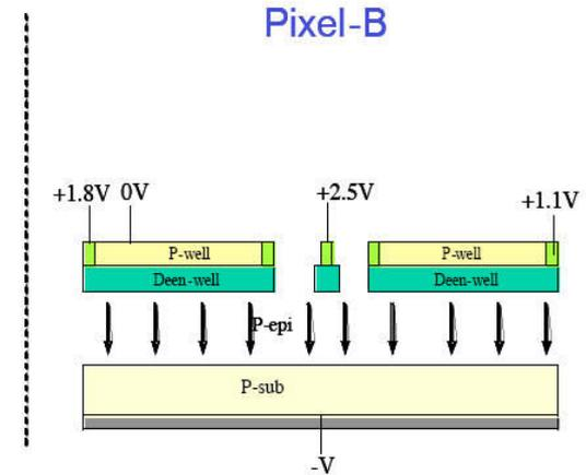
Figure 6.3 Comparison of the vertical cross section views of two pixels
