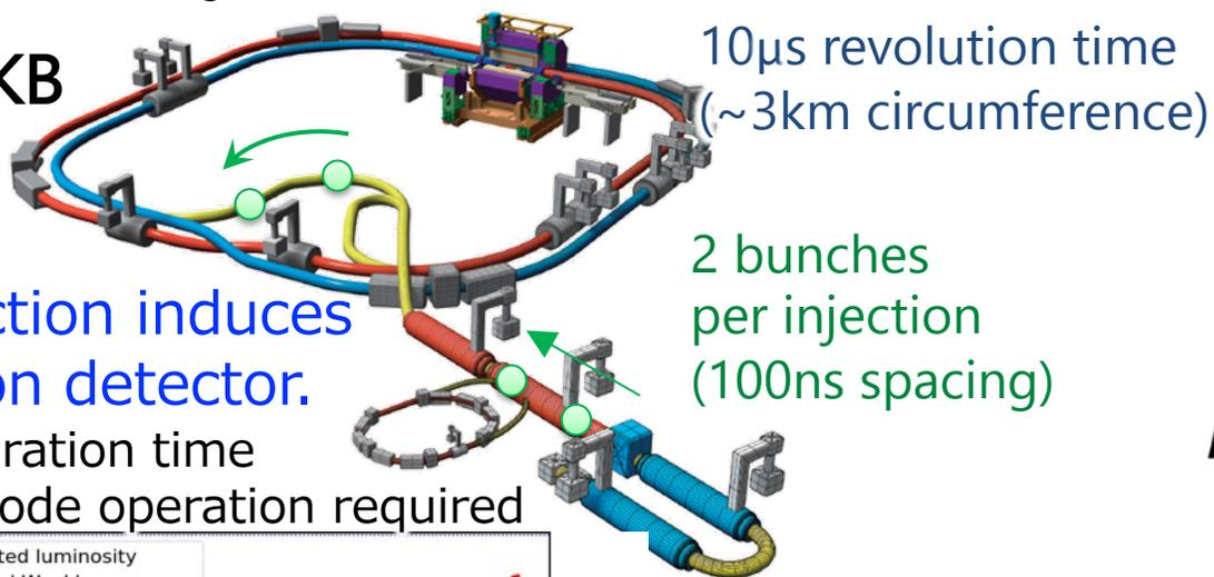
Every injection induces beam BG on detector.
