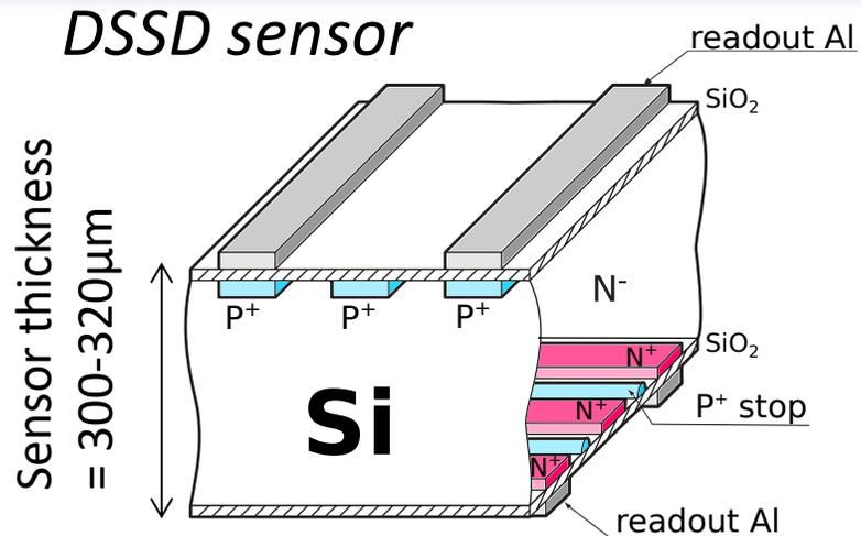
AC-coupled strips on N-type substrate
