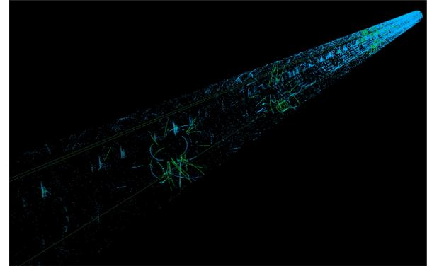
*TPC time frame visualization of real data from pilot beam*
