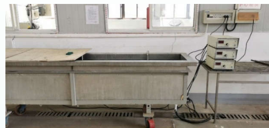
公司另配有超声波清洗仪3套 酸洗池1套 Ultrasonic cleaning device 3 sets Pickling tank 1set
