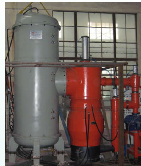
氢气/真空两用钎焊炉 \Phi 750 \times 3000 \text{mm} Hydrogen shielded/Vacuum brazing oven
