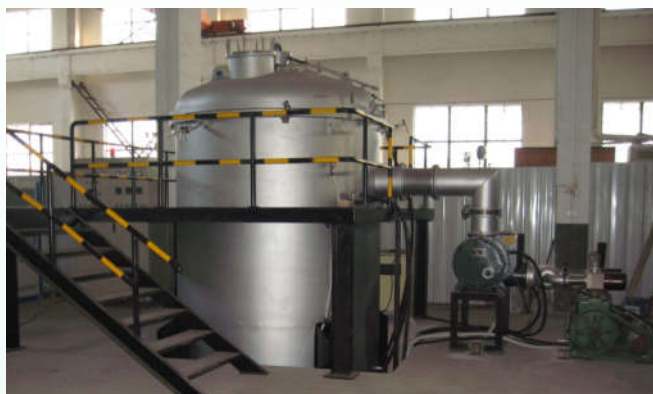
氢气保护钎焊炉 \Phi 1600 \times 2600 \text{mm} Hydrogen shielded brazing oven
