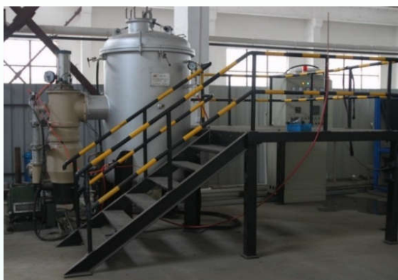
氢气/真空两用钎焊炉 \Phi 500 \times 1000 \text{mm} Hydrogen shielded/vacuum brazing oven
