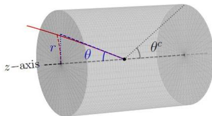
**Figure 2:** Skeleton diagram of a sideview of the TPC and a trajectory of one particle (marked by the solid red line) hitting its endcap, which has a  $p_T$  of 1.8 GeV/c and a  $\theta$  of 21°.
