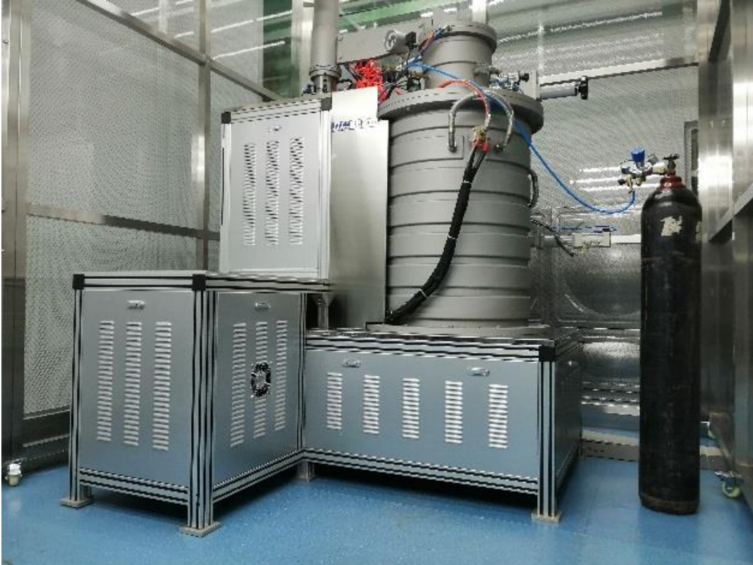
Furnace for Nb 3 Sn coating.
