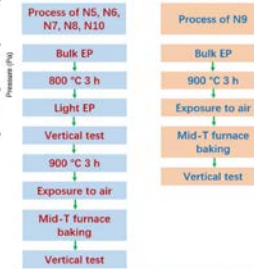
Treatments for 1.3 GHz 9-cell cavities mid-T furnace baked
