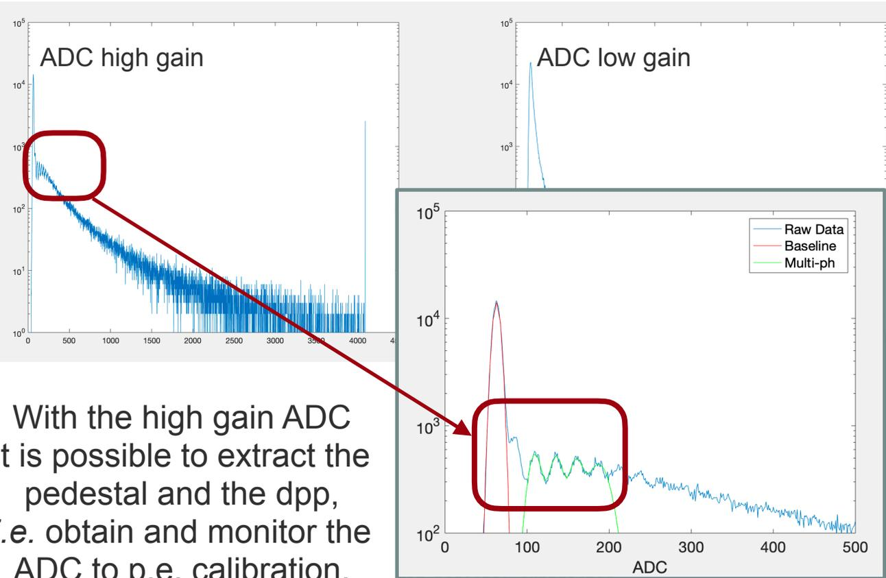
With the high gain ADC it is possible to extract the pedestal and the dpp, *i.e.* obtain and monitor the ADC to p.e. calibration.
