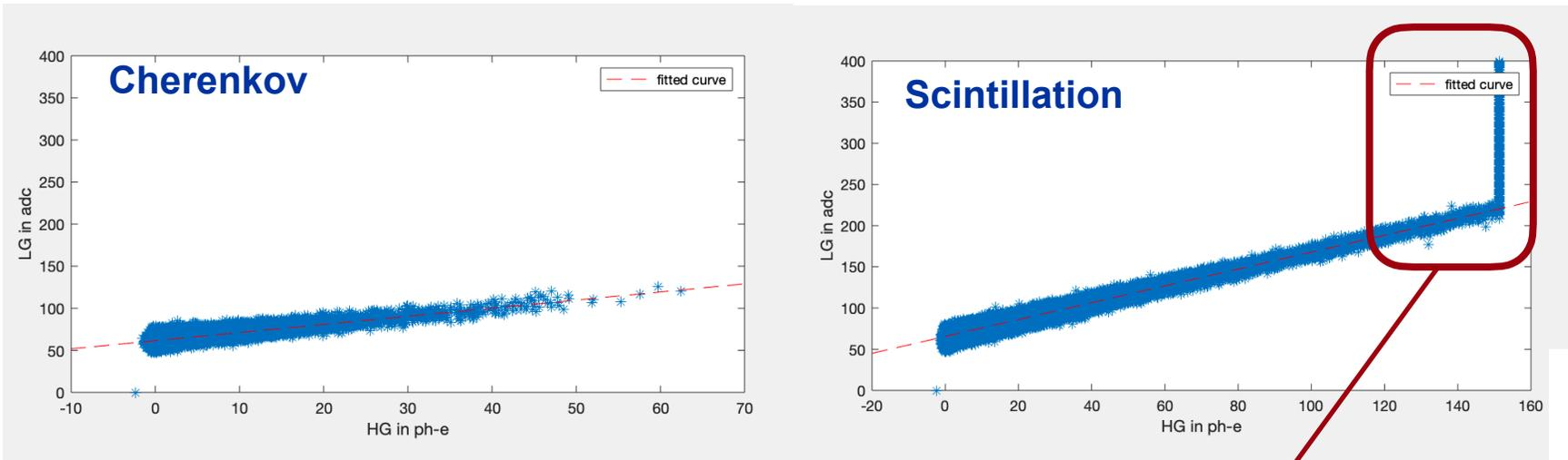
Reconstructed energy deposits for every SiPM obtained by combining the HG and LG signals.
