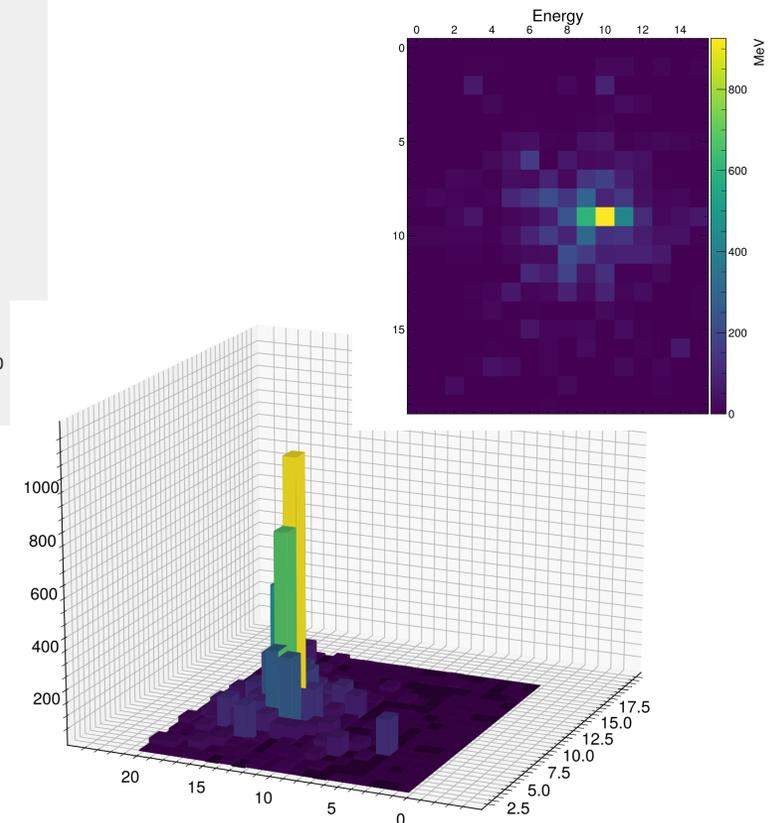
Clearly visible how the high gain saturation can be recovered.
