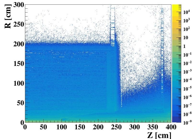
Charged particles fluence [Charged particles cm<sup>-2</sup>] for BX
