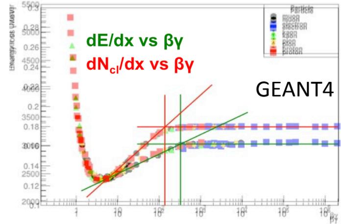
$dN_{cl}/dx$  Fermi plateau with respect to  $dE/dx$  is reached at lower values of  $\beta\gamma$  with a steeper slope
