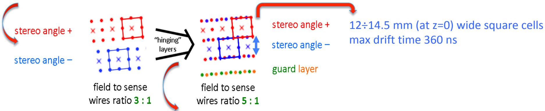
combination of + and - wire orientation produces a more uniform equipotential surface → 5:1 field to sense wires ratio (more field wires) → better E-field isotropy and smaller  $E \times B$  asymmetries )
