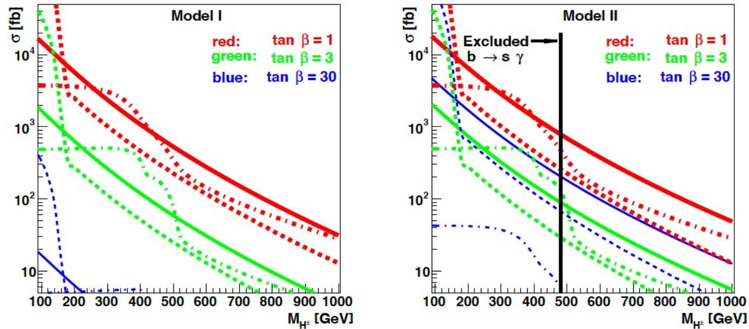
Figure 15: Charged Higgs production cross sections in the 2HDM, at 14 TeV. Left: Model I (or X). Right: Model II (or Y). Solid and dotted curves refer to “fermionic” channels, whereas dash-dotted refer to “bosonic” ones (see text).
