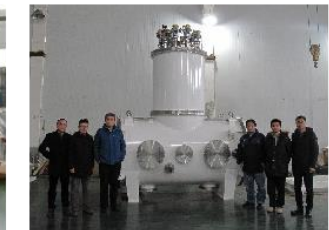
Horizontal test cryostat
