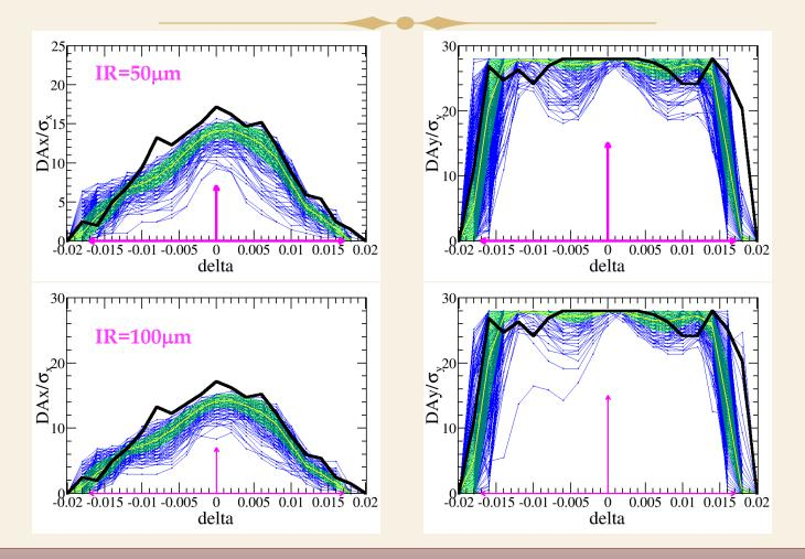
✓ The DA of 270 error seeds with errors ( = 100µm) satisfy the on-axis injection requirements.
