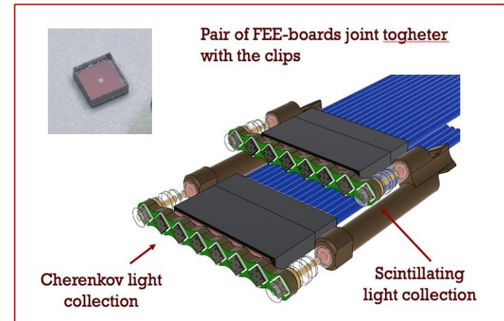
The SiPMs will be directly connected to the fibres and fixed to the absorber
