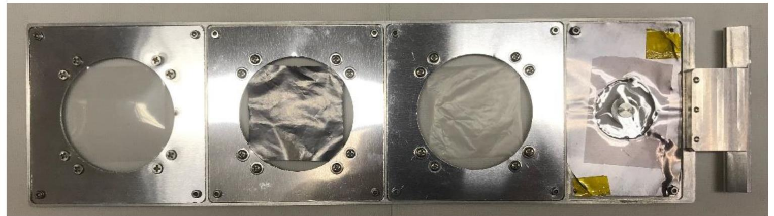
Fig. 1. The samples used in the present work. From left to right: \text{CH}_2 sample, graphite sample, \text{CD}_2 sample, and \alpha sources.
