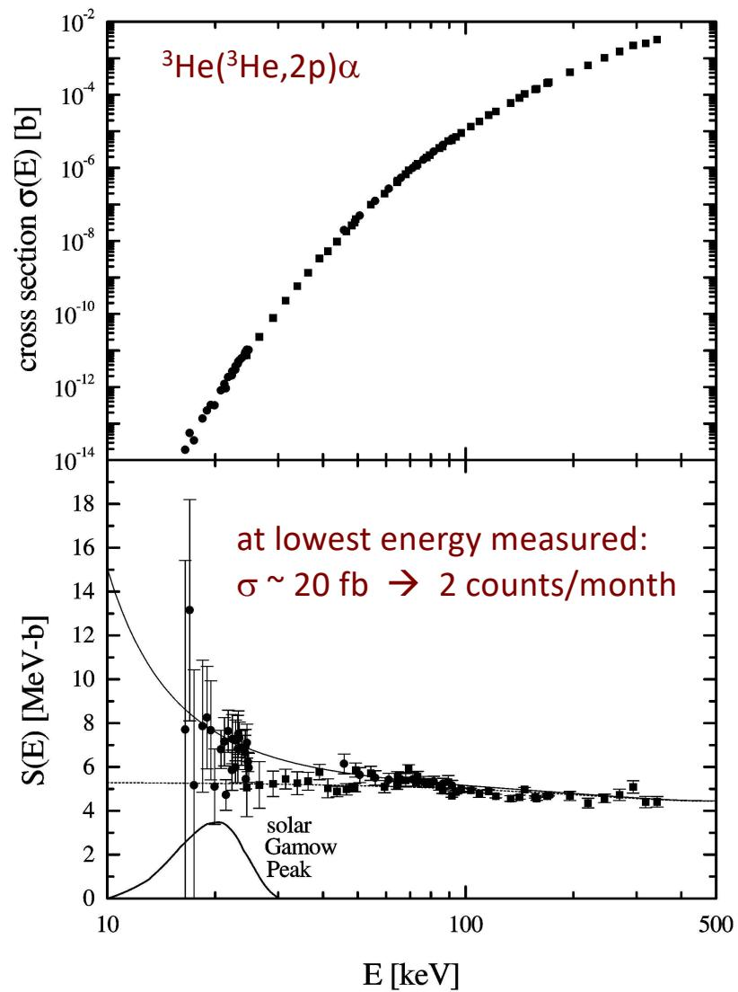
**First Measurement of the  ${}^3\text{He}({}^3\text{He}, 2p){}^4\text{He}$  Cross Section down to the Lower Edge
