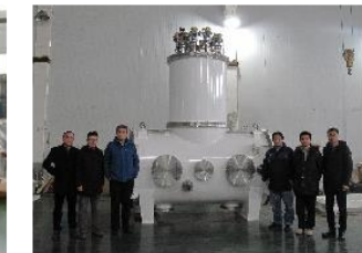
Horizontal test cryostat
