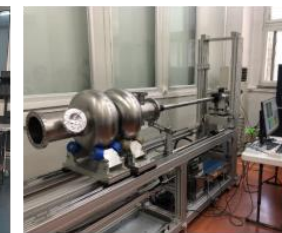
Cavity inspection camera and grinder
