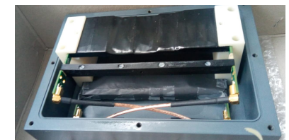
MEG2 scintillator tile read by SiPM
