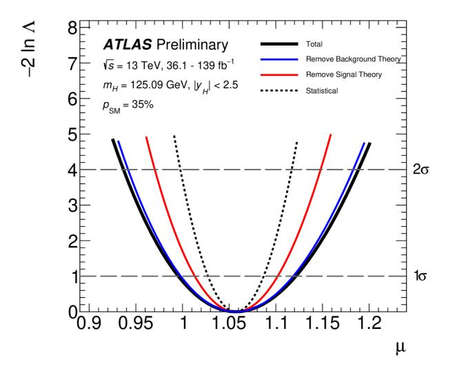
Inclusive signal strength, defined as the measured Higgs boson signal yield normalized to its SM prediction, is determined to be
