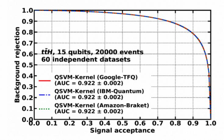
For 15 qubits, using ttH analysis dataset (20000 events), Google qsim simulator (red), IBM statevector simulator (blue), and Amazon local simulator (green) provide identical performances for QSVM Kernel method
