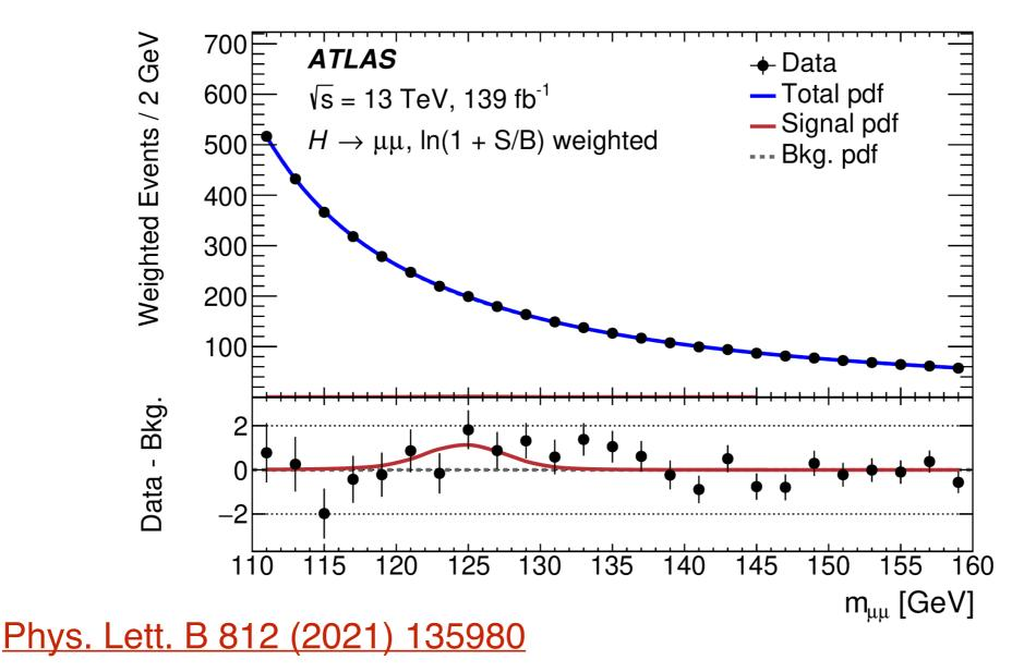
Dimuon mass spectrum: small excess at the Higgs mass around 125 GeV
