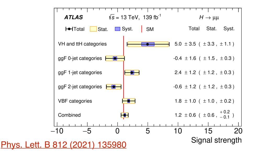
The measured H→µµ signal strength at 13 TeV is 1.2 +/- 0.6 (stat.) <sup>+0.2</sup>-0.1 (syst.)
