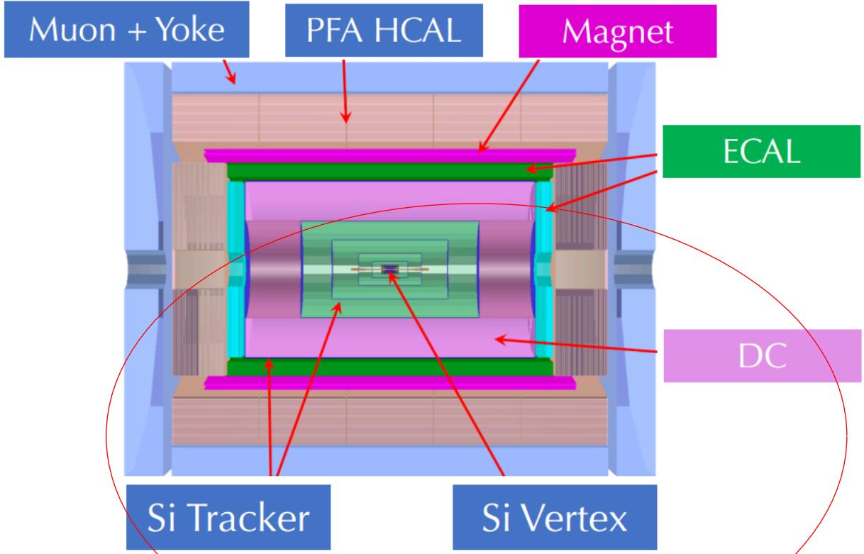
determine the preliminary layout of the tracker with fast method to get smallest resolution of helix parameters ( $d_0$ ,  $z_0$ ,  $\phi$ ,  $\theta$ ,  $P_t$ )
