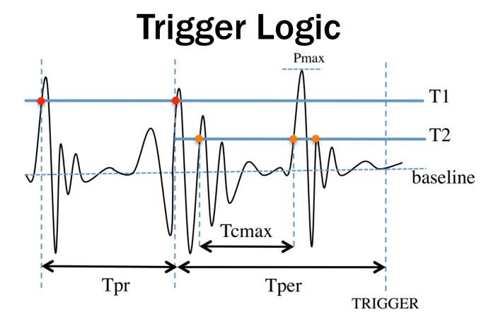
• Used to reject man-made RFI and capture radio pulses.
